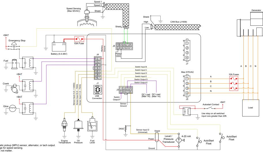
(1) Input is to be used for a magnetic pickup (MPU) sensor, alternator, or tach output.
